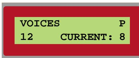
Nord Modular will always try to assign as many voices as you request. The current actual number of voices assigned is displayed to the bottom right in the DISPLAY. Note that voices will only be assigned to the selected SLOT(s) (SLOT LED lit or flashing). See [“Patch and voice allocation” on page 211](#) for more info.
