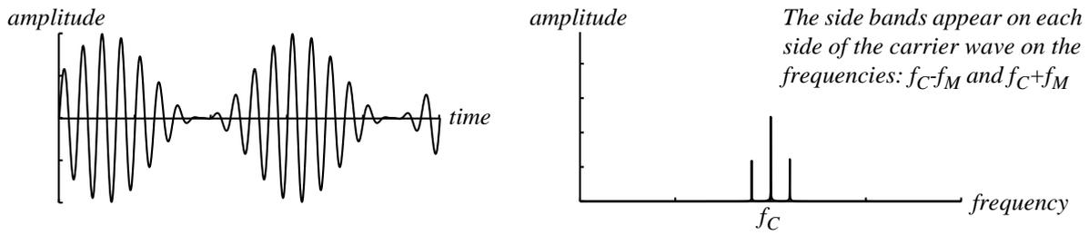
**Fig 3. Amplitude Modulation**
