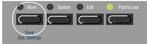
1. Activate a SLOT with a patch by pressing the SLOT button. If the EDIT or SYSTEM LED is lit, press the PATCH/LOAD button once. **You can not store any patches if Nord Modular is in System or Edit mode.**
