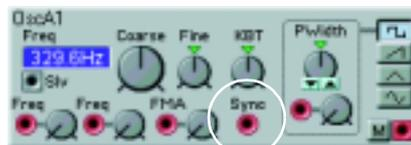
A waveform of an oscillator with a Sync input can be synchronized with a wave of another oscillator. The synchronization forces the wave to restart each time the modulating wave raises above 0. This results in a complex waveform that depends both on its own pitch and on the modulator pitch. When sync is used, the oscillator pitch is locked to the modulator pitch. If you change the modulator pitch, you will affect
