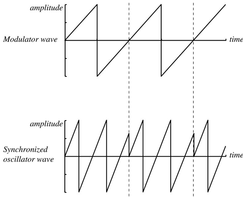
If you let the synchronized oscillator pitch vary continuously, from an LFO or other modulator, you will change the timbre of the wave in a very interesting and characteristic way.
