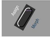
**SHIFT+ASSIGN** allows you to edit the Morph range of the parameter in focus (if it is assigned to a Morph group). Edit the Morph range with the **ROTARY DIAL**. See more about Morph in [“Morph groups” on page 40](#).
