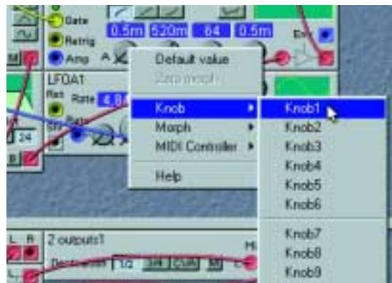
To deassign a **KNOB**, select Disable at the bottom of the popup menu. You can also re-assign a **KNOB** by selecting another (unused) Knob in the popup menu. This method also allows you to assign the other available, external controllers (Pedal, After touch and the On/Off switch) to a parameter. These controllers are found at the bottom of the Knob popup.
