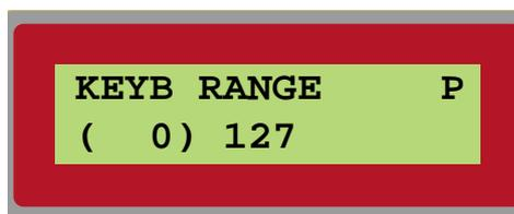
The patch will only receive keyboard information when you play within this range. If you want to use Nord Modular in a keyboard split situation, select two SLOTS, make sure that the Keyboard Mode is set to Selected Slots, and set the actual split point with the high key for one of the SLOTS and the low key for the other one.
