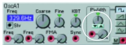
1. If you want to modulate the pulse width from the minimum value (1%) to the maximum value (99%) with a positive envelope (that produces a control signal with a peak to peak level swing from 0 units to +64 units), set the initial pulse width to 1% and the mod-amount to 127.
