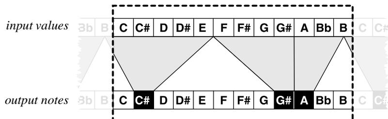
*Here we have activated the Cont function. As you can see, the input signal will be quantized to the selected notes in equal sections, per octave, across the selected range.*
