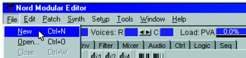
Select a slot in the dialog box that appears and click OK. This opens up a new, empty patch window in the Editor and clears the selected SLOT in Nord Modular. You can also choose not to select any SLOT by
