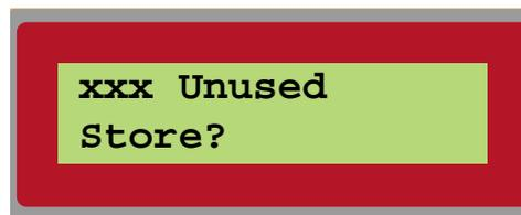
If you should run out of internal memory when trying to store a patch, this will be indicated by the following message in the DISPLAY:.
