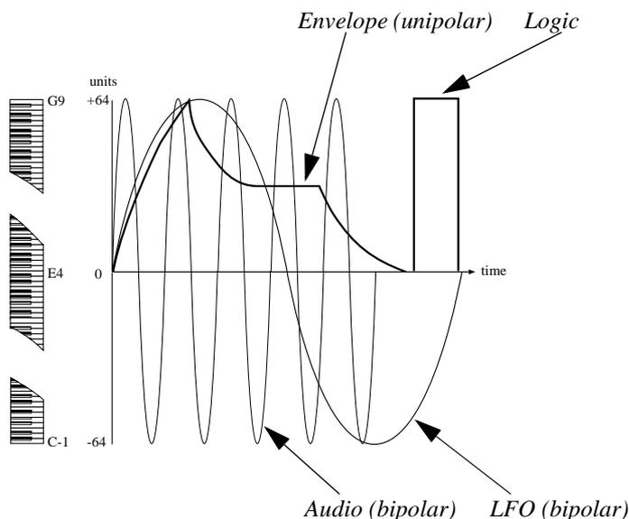
The LFO is an example of a bipolar modulator. Bipolar means that it sends both positive and negative levels (peak to peak -64 to +64 units). The keyboard is another example of a bipolar modulator. The key E4 (MIDI note number 64) represents 0 units in the Nord Modular system.
