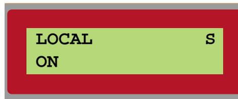
Select Local On to be able to control Nord Modular from the internal keyboard and the pedals. MIDI data is also transmitted via the **MIDI OUT** jack.
