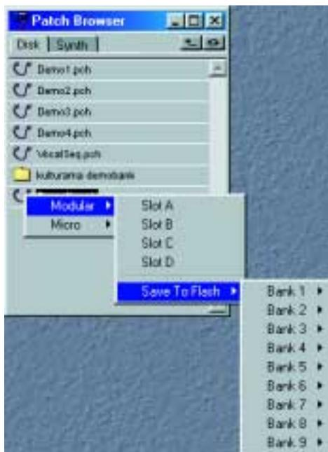
Here you can choose to either load the selected patch to any of the slots of the connected synthesizers and open the patch in the Editor patch window, or to save the selected patch in an internal memory location. The last function is exactly the same as storing a patch using the STORE button and the ROTARY DIAL on the Nord Modular front panel (see “Store” on page 50).
