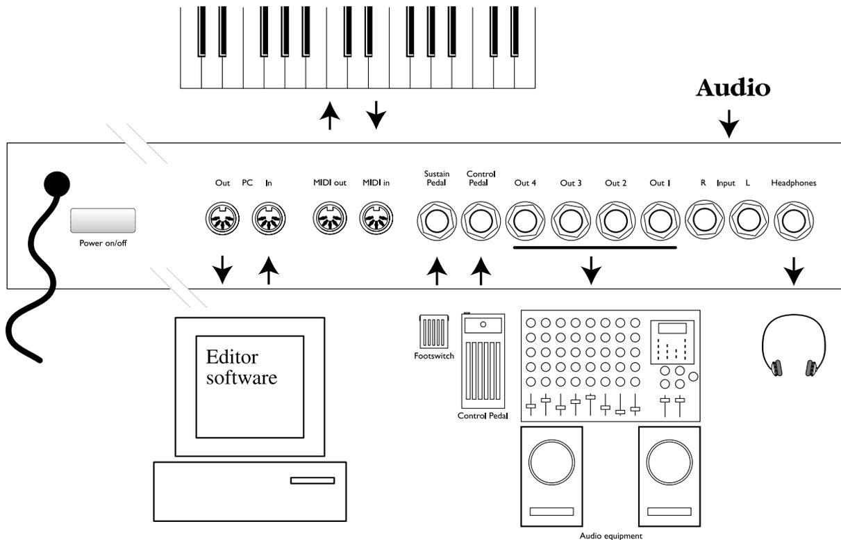
Use the **POWER ON/OFF** button to switch Nord Modular on and off.
