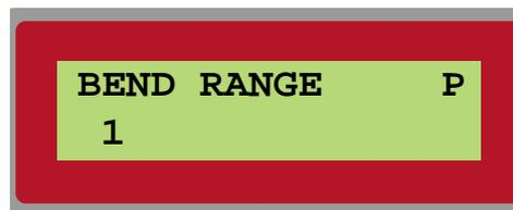
The pitch bend data will be added to the control signals from the Note outputs on the Keyboard modules and to the KBT (keyboard tracking) function. The range is from 0 to 24 semitones if KBT is set to 1. Oscillators, LFOs and filters using the KBT parameter will be affected by incoming pitch bend data.
