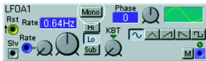
If you want modules in the Poly Voice Area of a polyphonic patch, e.g. one LFO per voice in a 4-voice patch, to be synchronized and behave like one single LFO, this can be done with the Mono parameter.
