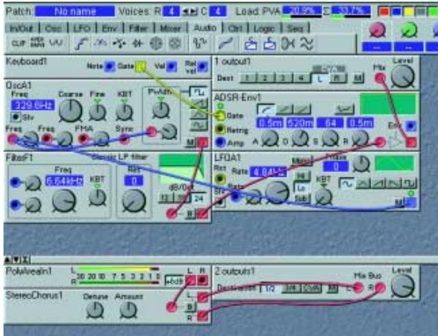
15. Finally, to make the patch editable and controllable from the Nord Modular front panel, you can assign any parameter in the patch to any of the 18 KNOBS of Nord Modular (3 KNOBS + 1 button on Micro Modular). Simply right[PC]/Ctrl[Mac]-click on a module parameter, for example, the Attack knob of the 'ADSR-Env' module, and select which KNOB to assign it to.
