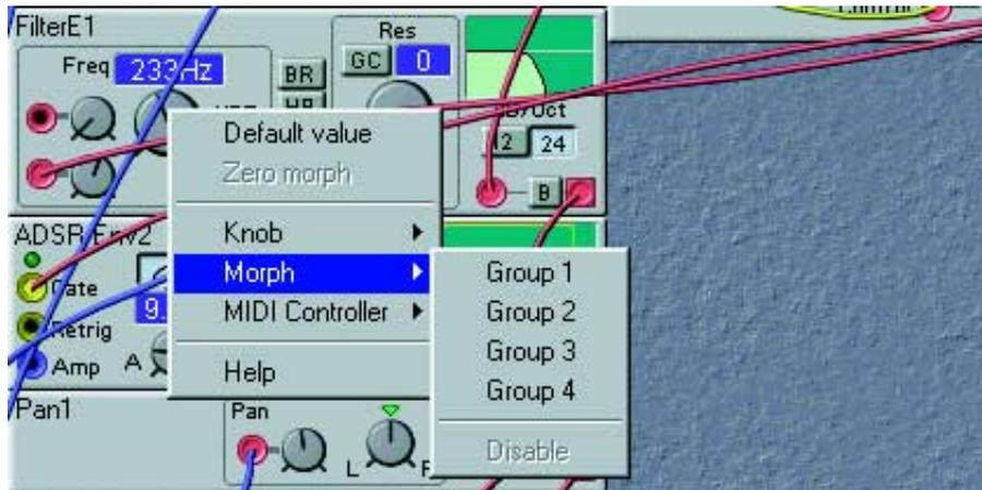
2. Every parameter assigned to a Morph group should also be given a Morph range. Click and hold the Ctrl[PC]/Alt[Mac] key on the computer keyboard and place the cursor on the knob that you assigned to the Morph group. Click-drag the cursor as if you were turning the knob. A colored sector will appear, indicating the Morph range. The range will also appear in a yellow hintbox above the parameter. You can also double-click-hold on a parameter that is assigned to a Morph group to set the range.
