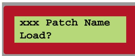
4. Load the patch by pressing the **PATCH/LOAD** button again. The patch is now loaded in the active slot. The number within parenthesis indicates the current polyphony of the patch.
