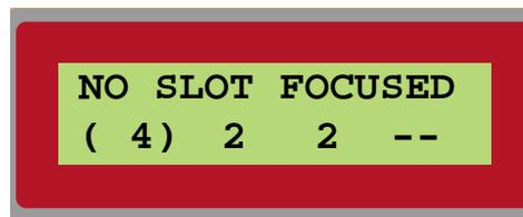
If several slots of the other Nord Modular are selected, but not active, you can still play one patch from the 2-octave keyboard (Nord Modular keyboard version). The patch played is that in the slot with the Current voice amount within parenthesis (slot A in this example).
