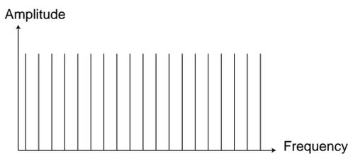
Let's now put this spectrum through a *lowpass* filter (this type of filter is discussed in more detail below). The filter has a characteristic, which can be shown as a curve in a frequency spectrum.
