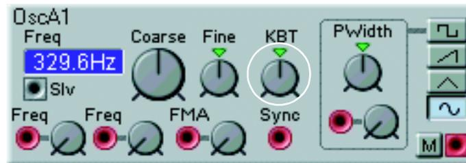
Any pitch bend appearing at the MIDI input will be added to the KBT tracking. Read more about scaling the pitch bend in [“Bend range” on page 57](#). If you, for instance, set up a sequencer patch, with KBT active on the oscillators, you can transpose the sequence in realtime by pressing keys on the Nord Modular keyboard. If any filters in a patch have the KBT parameter active, the cut-off frequency will also track the keyboard.
