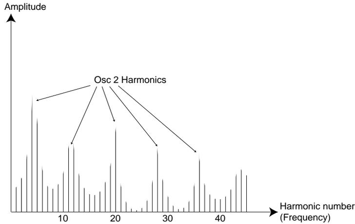
If you go even further and let the pitch of the synchronized oscillator vary continuously, for example from an LFO or envelope, you will change the harmonic content of the sound in an interesting and very characteristic way.
