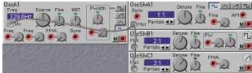
This signal is not particularly suited to connect to anything else in Nord Modular except another gray connector. The outputs are labelled “Slv” and the inputs are labelled “Mst”.
