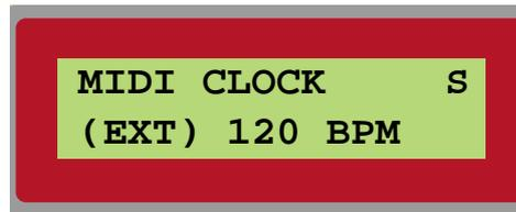
If EXT(external) is selected, any incoming MIDI clock can be used as a clock source in a patch. If INT is activated, the internal clock will be used. Navigate to the tempo indication and set the tempo with the ROTARY DIAL.
