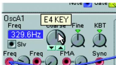
Press the EDIT button on the Nord Modular front panel (not Micro Modular). The parameter "in focus" in the Editor will also appear in the DISPLAY and you can now change the value of the parameter with the ROTARY DIAL.
