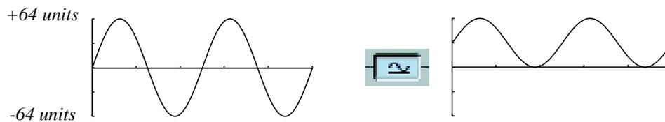
The left picture shows a bipolar control signal, and by clicking the Unipolar button, the signal becomes positive unipolar (the right picture)
