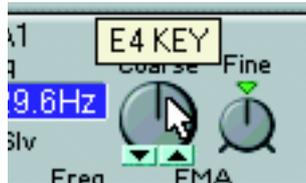
If Nord Modular (not Micro Modular) is in Edit mode (by pressing the **EDIT** button), the parameter will also be active in the Nord Modular **DISPLAY**, and you can adjust it with the **ROTARY DIAL**. You move the focus with the left and right **NAVIGATOR** buttons, or with the left and right arrow buttons on the computer keyboard, or by clicking with the mouse. The left and right **NAVIGATOR** and arrow buttons will only scroll through the parameters of one module.
