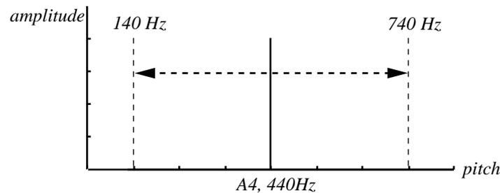
As you can see, FM modulation results in equal pitch shifting, in Herz, on either side of the basic pitch, whereas Pitch shifting results in equal shifting in the note scale.
