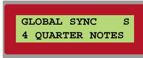
A setting of “4 QUARTER NOTES” will result in one logic Sync pulse for every 96 pulses from the Clock, which is equal to one pulse for every fourth quarter note.
