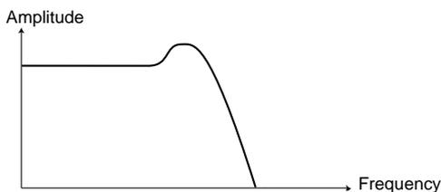
As you can see the curve is flat in the low register (which means it neither amplifies nor dampens the frequencies in this part of the spectrum) and then, at a certain point, gradually starts falling. When applied to the wave above, this filter cuts away some of the high frequency material in the wave, like this:
