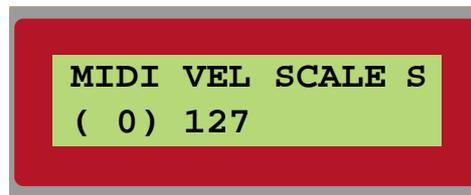
The number to the left is the minimum value and the number to the right is the maximum value. If your master keyboard transmits maximum velocity as 112, set the maximum value to 112. This ensures that the velocity response from Nord Modular will properly reflect the velocity transmission of the master keyboard.
