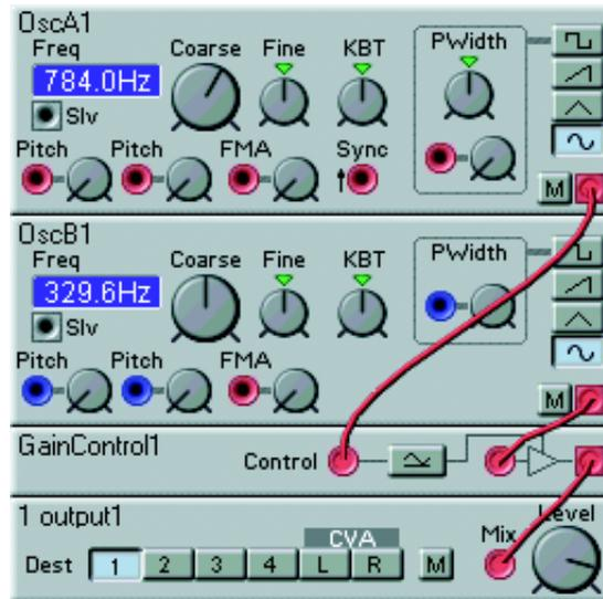
OscA is the modulator and OscB the carrier in this example. With the Unipolar button on the GainControl module not depressed, the setup functions as a ring modulator. With the Unipolar button depressed the setup works as an amplitude modulator.
