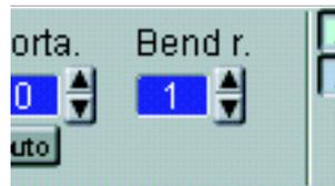
Here you set the range of the incoming pitch bend data in Semitones. The pitch bend data will be added to the control signals from the Note outputs on the Keyboard modules and to the KBT (keyboard tracking) parameter. The range is from 0 to 24 semitones. LFOs and filters that are using the KBT parameter will be affected by the incoming pitch bend data as well. Bend range can also be set in the Patch|Patch Settings dialog box (see [“Bend range” on page 68](#)).
