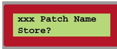
3. Select a Bank with the up/down NAVIGATOR buttons. Select a memory location with the ROTARY DIAL or with the left/right NAVIGATOR buttons and confirm by pressing STORE one more time. Pressing any other button will cancel the operation. It is possible to name your patch. The name can be set in the Patch menu (see [“Patch name” on page 57](#)).
