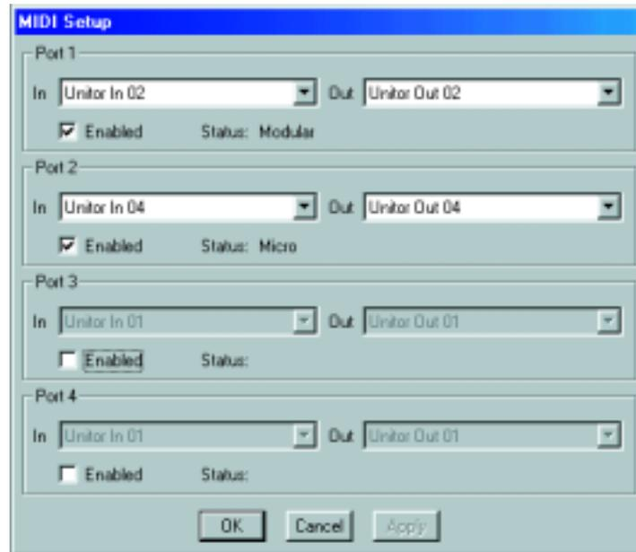
If the Nord Modular synth is not turned on, or if the connection between Nord Modular and the computer is not working properly, an error message will appear. In that case, check the MIDI connections and cables, make sure that the MIDI interface is properly installed and working, and that Nord Modular is turned on. Click on the Apply button. When the Editor has found the Nord Modular synth, the Name of the connected synth is shown in the Status line.
