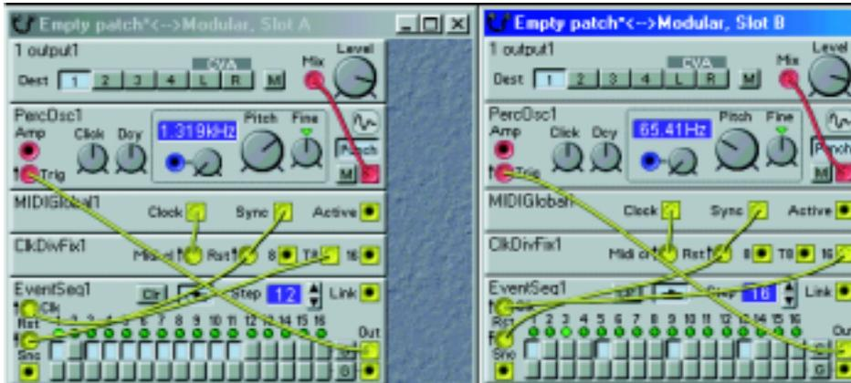
In this example, slot A is loaded with a patch performing triplets and the patch in slot B is playing quarter notes. Please observe the connections of the clock sources and the Rst signals.
