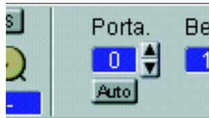
The portamento has two modes: Normal and Auto. In the Normal mode the portamento is always active, in the Auto mode you activate the portamento by playing legato. With the up and down buttons you set the time it should take to reach the new note.
