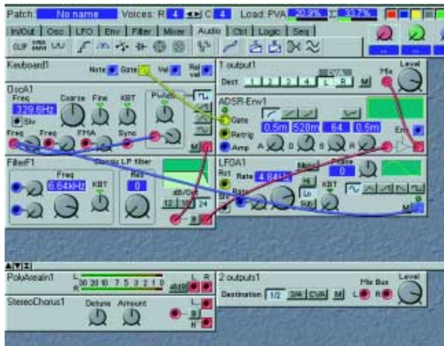
14. Now, connect the red L audio output of the 'Poly Area In' module to the red circular input of the 'Stereo chorus' module. Then, connect the two outputs of the 'Stereo chorus' module to the inputs of the '2 Outputs' module. As you play, you can see the LED chain of the 'Poly Area In' module display the signal level from the Poly Voice Area. If you need to, increase the level on the '1 Output'
