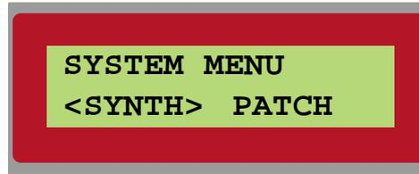
As mentioned above, the Synth Settings are global. To alert you that you are editing Synth Settings, an S is always shown in the upper right corner of the DISPLAY. Navigate between the sub menus with the up/down NAVIGATOR buttons and within the sub menus with the left/right NAVIGATOR buttons. Enter data with the ROTARY DIAL.
