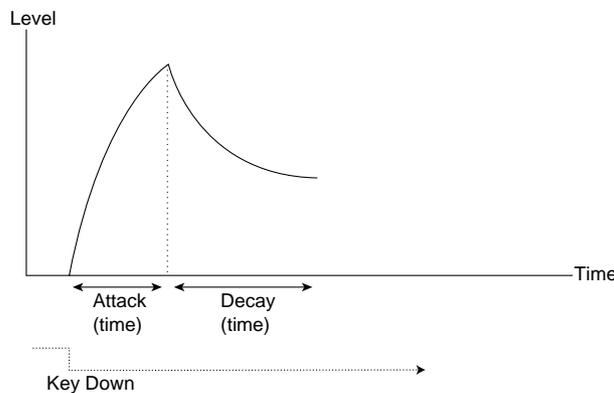
The level of the envelope does not necessarily have to fall all the way back to zero at the end of the decay. Instead, the ADSR-envelope has a *Sustain* setting used to determine the level the envelope should rest at, after the decay. If you for example want to create a flute sound, you would have a fairly high sustain setting on your volume envelope, since a flute tone basically stays at a steady level for as long as you play it.
