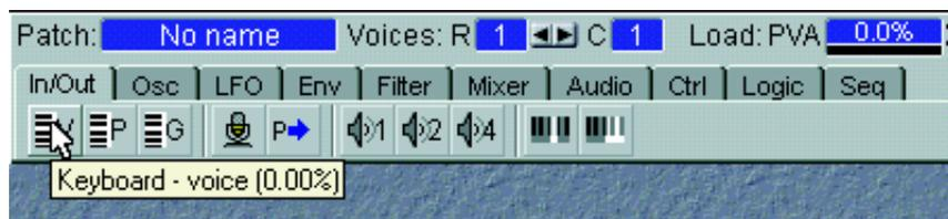
Select a group tab, click-hold on a module icon and drag it to the patch window. When you place the cursor over any of the module buttons, a brief description of the module appears together with information of the amount of patch Load (Sound engine power) it will use (PC version only).
