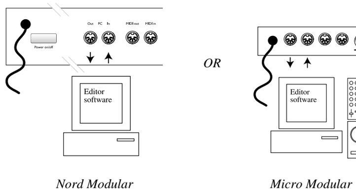
**Note! You cannot use the Editor software and the Nord Modular PC ports in a traditional MIDI set-up, using MIDI THRU-boxes or MIDI THRU connections on other instruments. The Nord Modular PC ports have to be used exclusively for the Editor software on the computer.**
