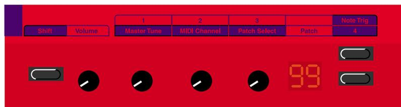
The **SHIFT** button activates a secondary function on some buttons and knobs.
