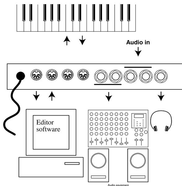
Connect the MIDI Interface of the computer that runs the Editor software to the **PC IN** and **PC OUT** ports. Connect any external MIDI equipment to the **MIDI IN** and **MIDI OUT** ports. This could be a sequencer, a master keyboard or another MIDI device.
