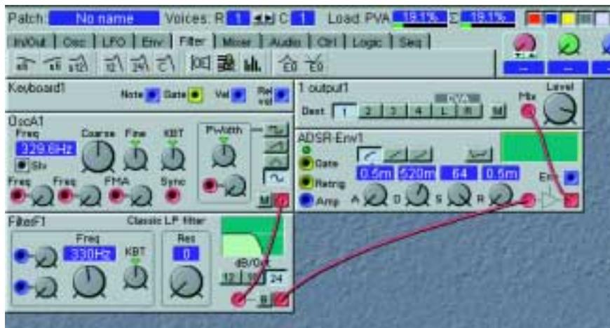
10. Even though all audio cables have been properly connected, no sound is heard. You have to make the envelope generator "open up" for the audio signal. Place the cursor on the yellow Voice gate output
