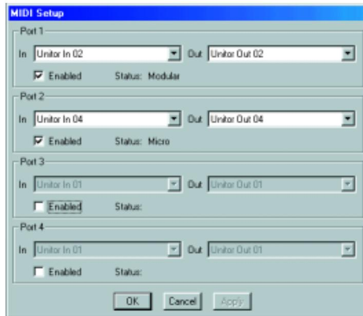
Place a check in the Enabled box for each connected Nord Modular synthesizer and select a MIDI port from the drop-down menu(s). Click on the Apply button. When the Editor has found the Nord Modular synth(s), the Name of the connected synth(s) are shown in the Status line. When you're satisfied with the port selection, click OK. (It isn't necessary to click Apply before clicking OK. You can click OK directly after having enabled and selected the ports, but this will close the dialog box.)
