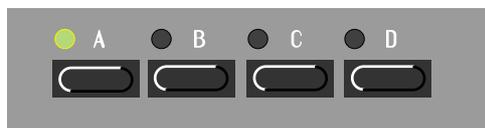
If several slots are selected, by simultaneously pressing several **SLOT** buttons, a solid green LED will indicate a selected slot and a flashing LED will indicate the currently active **SLOT**. Every selected **SLOT** will receive MIDI messages on their set channels, but only the active **SLOT** will transmit MIDI messages.
