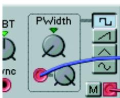
2. If you want to modulate the pulse width from the minimum value (1%) to the maximum value (99%) with an LFO (that produces a bipolar control signal with a peak to peak level swing from -64 units to +64 units), set the initial pulse width to 50% and the mod-amount to 64.
