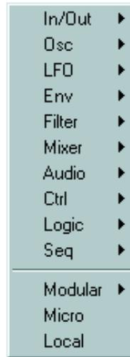
Select desired module by clicking on it from the list. A phantom frame appears and the cursor gets a plus-sign next to it. Place the phantom frame where you want the module to be placed and click to drop the module.
