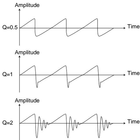
If you add resonance to a sound and then vary the Cutoff frequency (for example with an envelope) you will get a very typical synthesizer sound.
