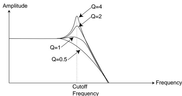
High resonance values are also visible in the waveform. They appear as a “superimposed” waveform with a frequency equivalent to the filter’s cutoff frequency. The three examples below show the same wave with increased resonance.
