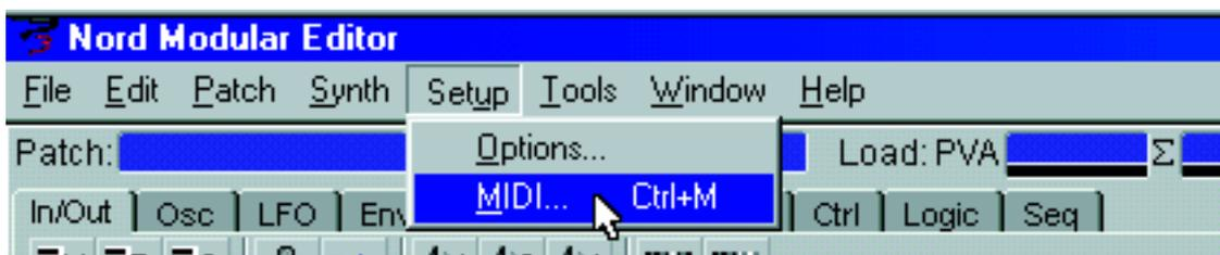
Check in the Enabled box for Port 1. If the MIDI interface driver(s) have been properly installed, you will be able to select a MIDI port in the In- and Out dropdown lists. Up to four Nord Modular synthe-
