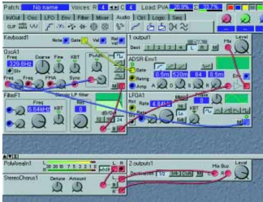
The '1Output1' module in the Poly Voice Area is set to route the signal to CVA L, the left output of the 'PolyAreaIn1' module in the Common Voice Area. The sum of all voices from the Poly Voice Area is sent to the Common Voice Area to be processed in the 'StereoChorus1' module and output at OUT1 and OUT2 jack of the synthesizer.
