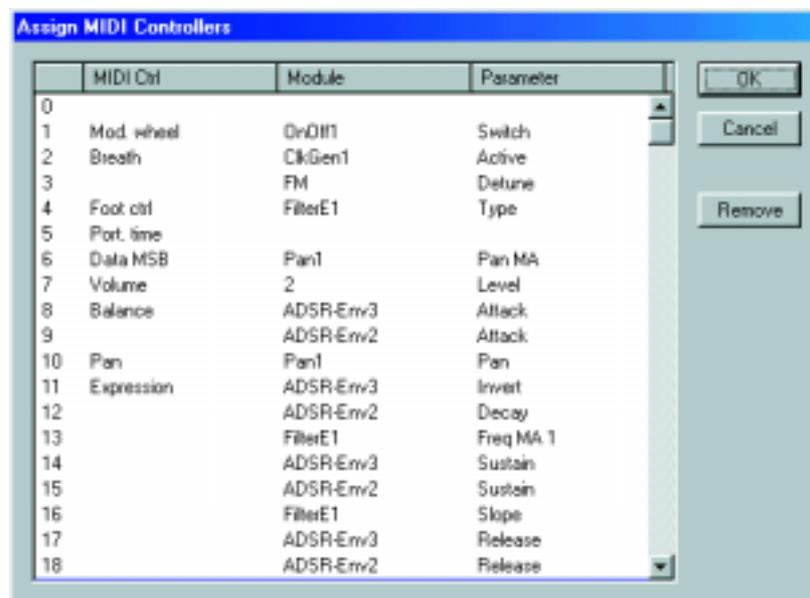
Some of the MIDI Controllers usually have designated functions, like Controller 1, Mod Wheel. These designated Controllers are just numbers to Nord Modular. You are free to assign up to 119 MIDI Controllers to module parameters. MIDI Controller #32 (Bank Change) and #64 (Sustain Pedal) cannot be selected from this list. If you want to control external MIDI devices, these labels may have greater importance.
