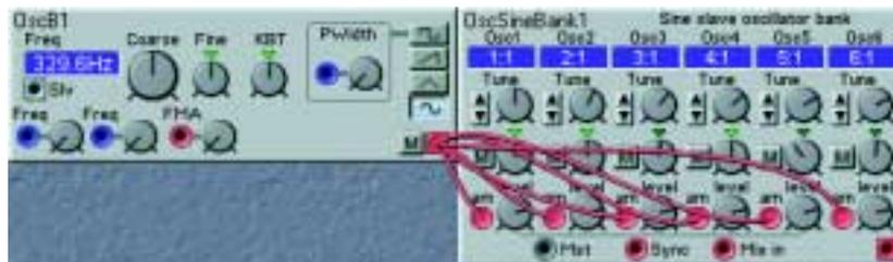
You can also make a serial connection, from input to input, provided that the first input in the chain is connected to an output. The result is exactly the same as in a branch connection. If a module within a serial cable chain is removed, the remains of the cable chain will be re-routed.
